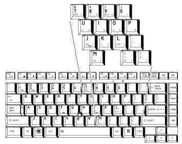
Figure 5-2 The numeric keypad overlay
